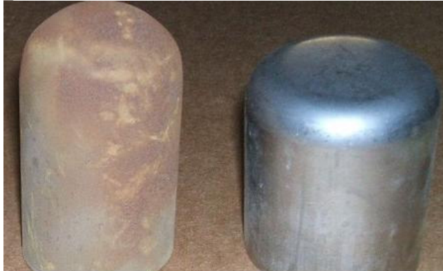
Some have rust on them and some are clean. You can use Emery cloth /sand paper to clean
